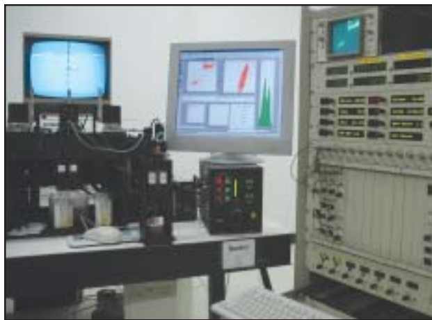
A flow cytometer is the machine that sorts semen into X-bearing semen and Y-bearing semen after it has been stained with fluorescent dye.
